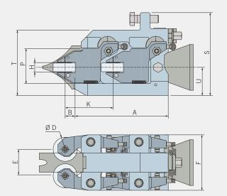
Guide setting tools. Guide setting on workshop and alignment on the mill with standard optic devices or with computerized HiLINE.
